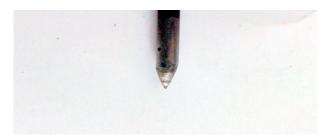
a The conventional TIG electrode with diameter 2.4mm
