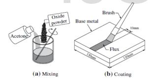
Fig 1. Schematic diagram of activated TIG welding
