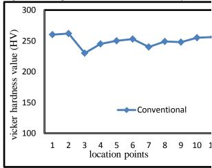
Fig.6 Micro hardness profile across the weldment for Conventionl TIG
